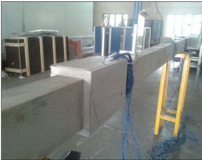
Fig. 2: Mounting of the Sandwich Busduct on steel stands.
